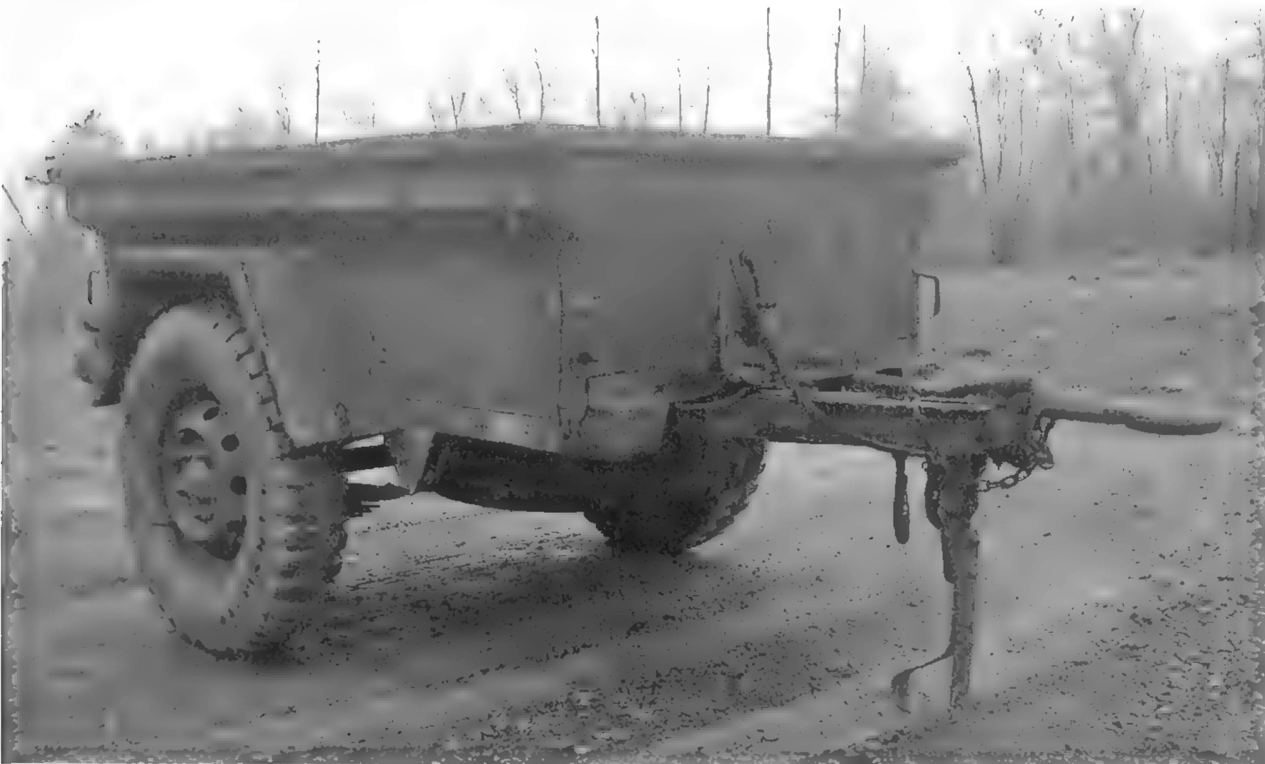
The M416 was slightly wider than its predecessor trailers, but the quickest way to distinguish it is the flat-topped angular fenders. This trailer has been modified with a spare tire under the bottom, and a flat steel cover over the cargo area. (Photo courtesy of TacticalTruck.com)
